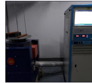
Gift Box Packaging Vibration Test
